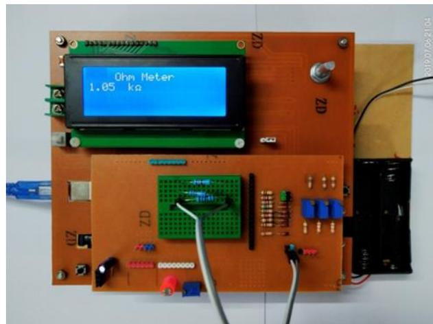
**Figure 8:** Photograph of measuring results for resistance circuit
