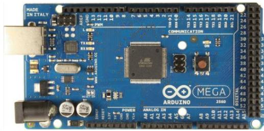
**Figure 1:** The component of Arduino mega 2560 microcontroller
