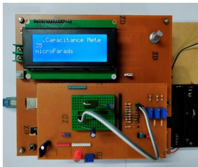
**Figure 9:** Photograph of measuring results for capacitance circuit
